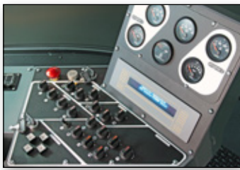
Electronic Monitoring and Control System (ECS) and operator's console
