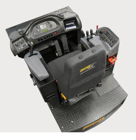
Equipment Management Monitoring System - mounted in front of the operator for easy viewing of gauges and warning lights
